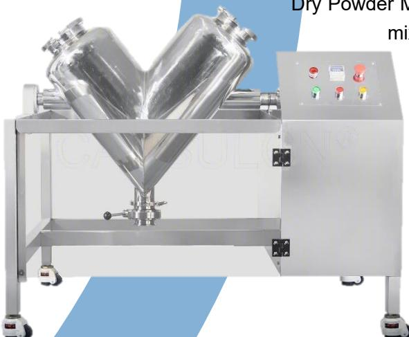
Dry Powder Mixer Blending Machine Mixer V50 Pro (with protective fences) is a mixing machine from CapsulCN. It is suitable for mixing various dry powder and granular materials in pharmaceutical, chemical and food industries. The mixer has characteristics of simple structure, easy operation and pretty appearance. Its parts in contact with materials are made of stainless steel, which conforms to the CGMP.
