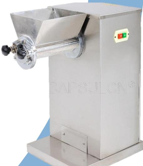
This machine is used mainly in such trades as pharmacy, chemical industry, food, pottery and plastics extensively, making moist powder material particle. Make cylinder swing reciprocally, extruding material from screen mesh for granulation. It also can be used for crushing the agglomerate materials into small granules directly.
