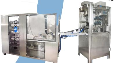
As a market leader in liquid-fill technology, we have taken extra care to ensure proper filling of liquids. The NSF capsule sealing machine seals the cap and the body of the capsule at high speed.
