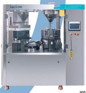
Cap**CN**-72/240 automatic capsule filler processes the products for optimal productivity up to 1200/4000 capsules per minutes, featuring low-maintenance operation, minimal downtime, and overall dependable production.
