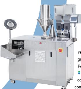
This machine adopts programming control system, touch panel operation, stepless frequency conversion speed regulation, pneumatic joint control, and electronic automatic counting device, which can automatically complete the capsule positioning, separation, filling, locking and other actions.
