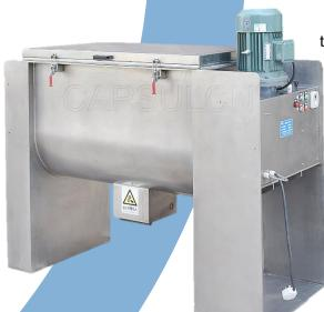
Ribbon Blenders consist of a U-shaped horizontal trough, transmission parts and ribbon agitating blades which usually have double or triple layers with outside screw gathering the material from sides to center and inside screw transmitting the material from center to sides to form convection mix and a specially fabricated ribbon agitator.
