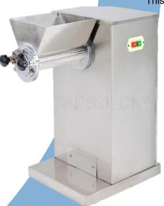
This machine is used mainly in such trades as pharmacy, chemical industry, food, pottery and plastics extensively, making moist powder material particle. Make cylinder swing reciprocatly, extruding material from screen mesh for granulation. It also can be used for crushing the agglomerate materials into small granules directly.
