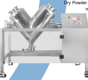
Dry Powder Mixer Blending Machine Mixer V50 Pro (with protective fences) is a mixing machine from CapsulCN. It is suitable for mixing various dry powder and granular materials in pharmaceutical, chemical and food industries. The mixer has characteristics of simple structure, easy operation and pretty appearance. Its parts in contact with materials are made of stainless steel, which conforms to the CGMP.
